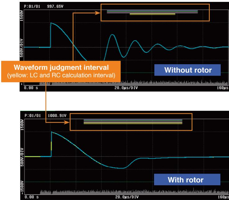
When a rotor is present, the ST4030A reduces the amount of electrical energy supplied to the motor, causing attenuation of the response waveform.
