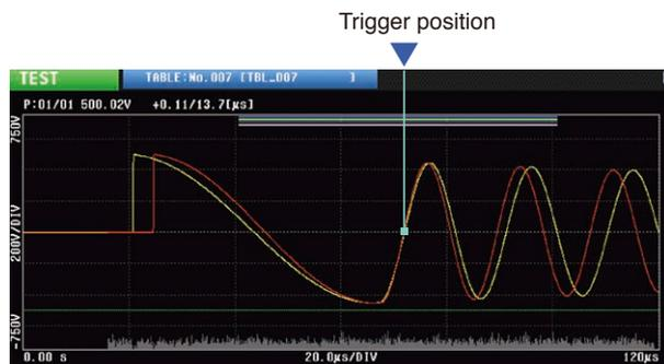
Make judgments based the response waveform using the second waveform, where characteristics unique to the workpiece being tested most readily appear, as the trigger.
