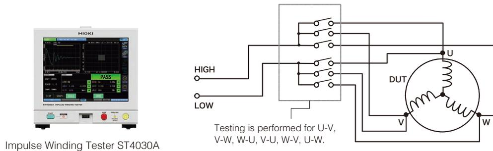
Automate testing using a setup such as the one shown below by using a High Voltage Scanner 3930 to switch the measurement circuit.
