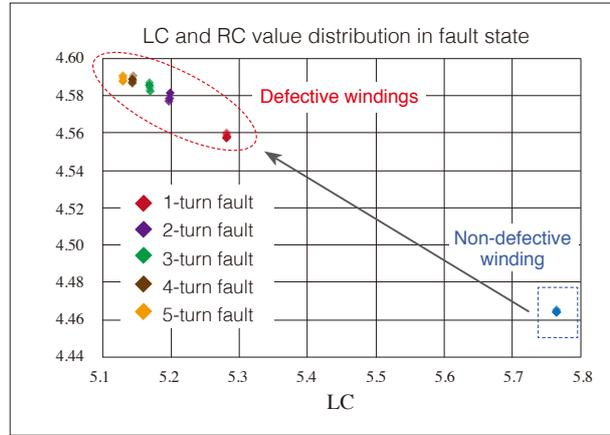
**The distributions of values differ for defective and non-defective windings.**
