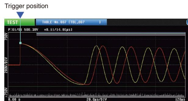
Make judgments based on the response waveform using the rising edge of the application waveform as the trigger (the same approach used by conventional testers).
