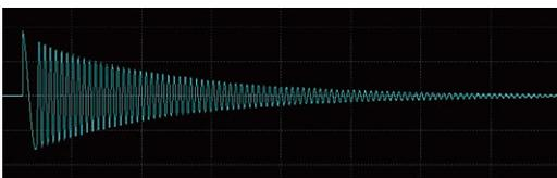
An unnecessary amount of waveforms is being captured due to the response waveform's high oscillation frequency. Either the sampling frequency needs to be increased, or the sampling data count needs to be decreased.
