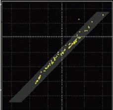
Select when the motor's rotor has been attached and the distribution of the LC and RC values assumes a belt shape according to the rotor position or angle
