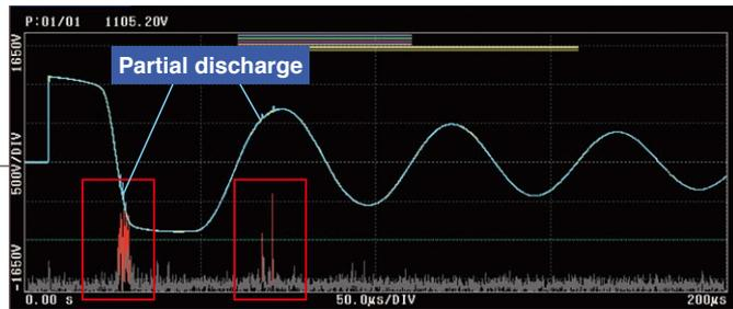
High-frequency discharge components are isolated by a proprietary Hioki filtering process.
