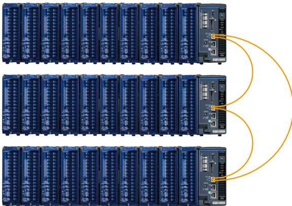
Example of synchronized measurement with 3 loggers
