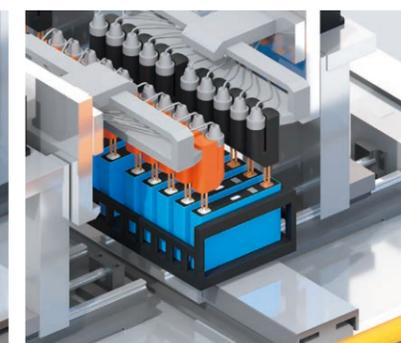
Testing of prismatic cells
