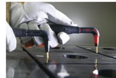
L-shaped lead for measurement in confined locations.
