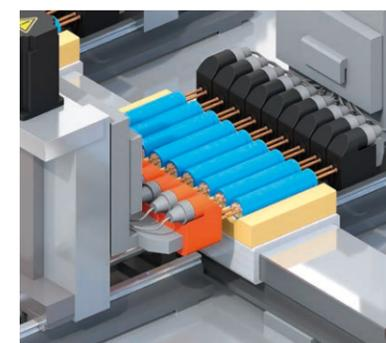
Testing of cylindrical cells
