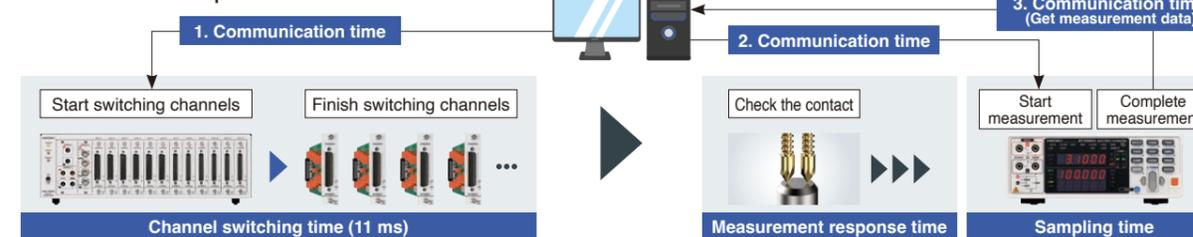
$$\text{Cycle time calculation} \quad \text{Total time} = (\text{Communication time} + \text{Channel switching time} + \text{Measurement response time} + \text{Sampling time}) \times \text{Number of channels}$$
