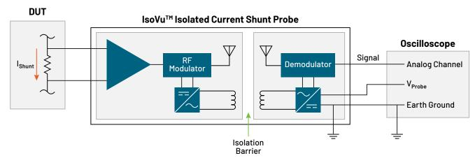
Complete galvanic isolation between the probe tip and the oscilloscope eliminates ground loops and delivers extraordinary common mode rejection.
