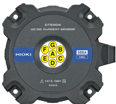
When using sensors designed to take into account the effects of conductor position, changes in conductor position have only a small effect on the measured value.
