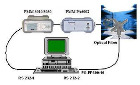
Fig. 3-3 PMM EP-600/601/602/603/604 in Anechoic Chamber
