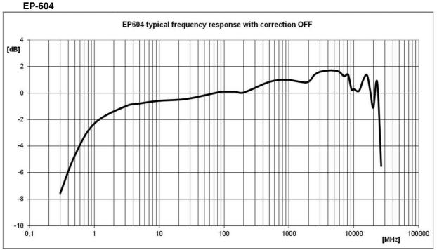
Fig. 1-10 EP-604 typical frequency response with correction OFF
