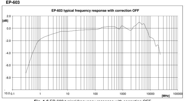
Fig. 1-6 EP-603 typical frequency response with correction OFF
