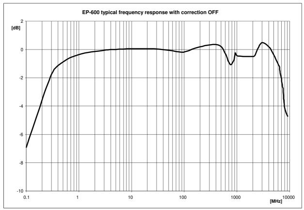
Fig. 1-3 EP-600 typical frequency response with correction OFF
