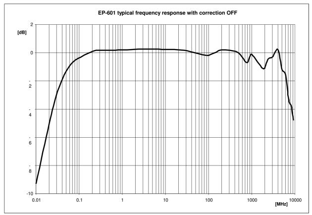
Fig. 1-4 EP-601 typical frequency response with correction OFF
