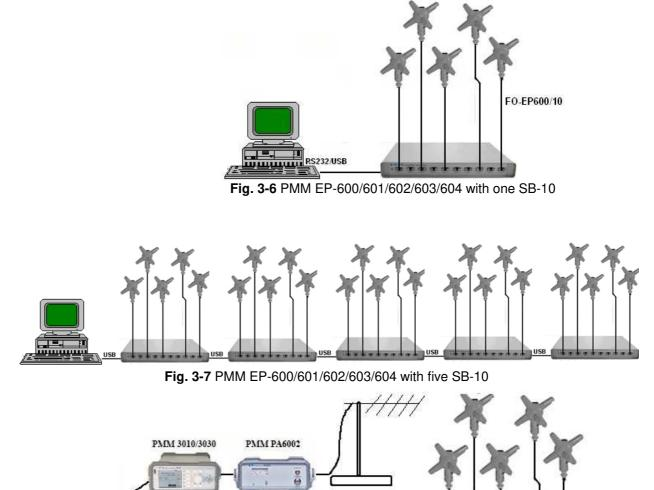
Fig. 3-8 PMM EP-600/601/602/603/604 with SB-10 in open site
