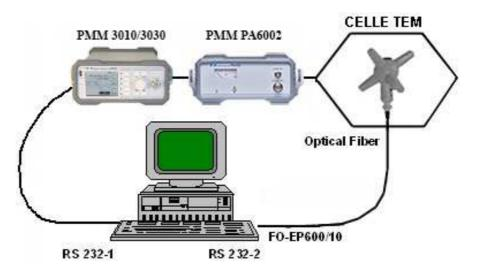
Fig. 3-2 PMM EP-600/601/602/603/604 in TEM cell
