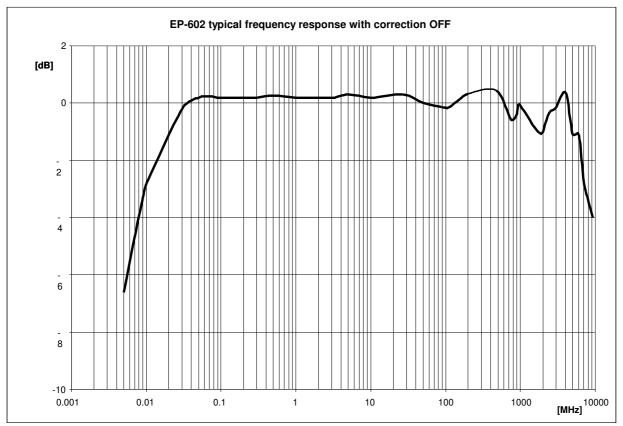
Fig. 1-5 EP-602 typical frequency response with correction OFF
