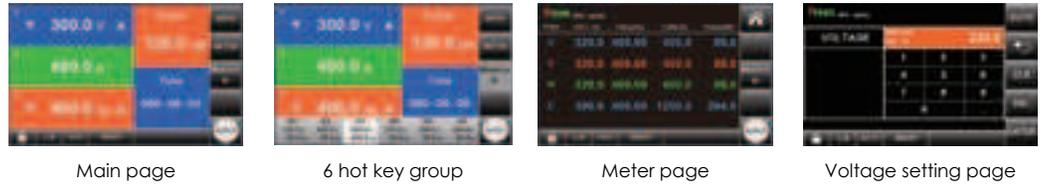
The new AFC series has updated with an enlarged touch screen that can make fine tune adjustment for parameters and changing values. With RS-232,RS-485 interface, AFC is able to be controlled remotely. The colorful display allows user to quickly recognize all the parameters including voltage, current and PF with 6 groups of hot key that can promptly switching at a glance.
