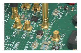
IsoVu probe tips have a range of connections and accessories that offer high performance and accessibility. The probes can connect directly to MMCX connectors, which are inexpensive and widely-available. This makes for stable, hands-free test points and offer high bandwidth and common mode rejection. The solid metal body shields the center conductor and minimizes ground loop area for the lowest interference possible.
