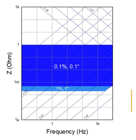
EIS CONTOUR MAP The system has been optimized for EIS measurements of pouch and prismatic cells.
