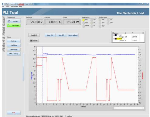
Measurement values of the internal DAQ memory can be exported from the electronic load and displayed as a diagram with the aid of the "Data Viewer". The measurement data can also be saved on a data storage as a .CSV file for further processing.
