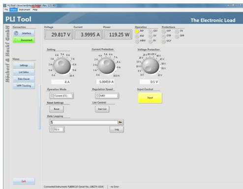
The PLI software tool is a graphical software tool to control the PLI series electronic loads. The user can choose different functions with the aid of the navigation bar.
