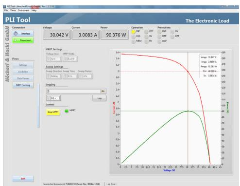
The MPPT function acquires measurement data from a connected solar panel. The function changes continuously between the MPPT process and a sweep process. During the MPPT process, the load controls the optimum global MPP found at the sweep process.
