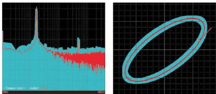
Judge FFT analysis waveforms and X-Y waveforms by area
