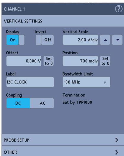
Configuration menus are accessed by simply double-tapping on the item of interest on the display. In this case, the Channel badge was double-tapped to open the channel configuration menu. Menus are dismissed by simply tapping outside of them.
