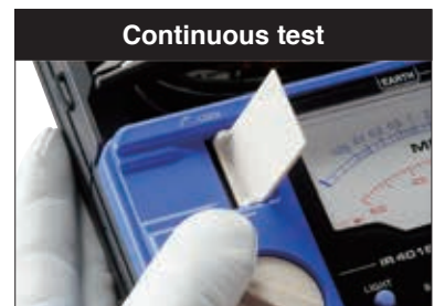
Lift and lock the MEASURE key to apply a continuous stream of voltage
