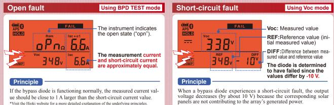
By detecting this difference, it is possible to detect bypass diode short-circuit faults and cell string losses.
