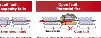
When an open fault occurs, current is forced to flow to the defective cell when it's covered by a shadow, causing the panel to heat up and posing the risk of fire.
