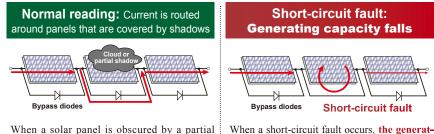
shadow (or when it fails), the current bypasses ed current flows in a loop, making it impossithe panel in order prevent any drop-off in genble to capture the generated power, resulting in lowered efficiency.
