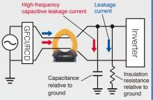
Measure leakage current at frequency characteristics that approach those of the GFCI or RCD
