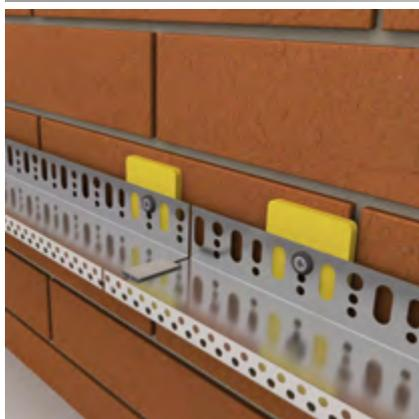
**Spacer** for levelling the substrate on the spot of anchoring a base profile with a hammer-in anchor in the thermal insulation system - ETICS
