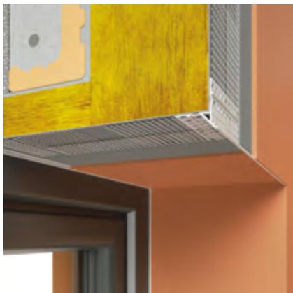
**LTDU window drip bead** with invisible drip-edge (hidden under plaster) and glass fibre mesh for finishing plasters and water drainage at the window heads in the thermal insulation system - ETICS. The bead can also be used as a balcony drip bead. The bead can also be at the bottom edge of the system where the LO base profile is not used for the insulation layer set-up
