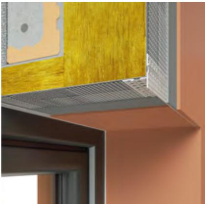
**LTU window drip bead** with invisible drip-edge (hidden under plaster) and glass fibre mesh for finishing plasters and water drainage at the window heads in the thermal insulation system - ETICS. The bead can also be used as a balcony drip bead. The bead can also be at the bottom edge of the system where the LO base profile is not used for the insulation layer set-up
