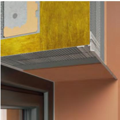
**LTHU window drip bead** with invisible drip-edge (hidden under plaster) and glass fibre mesh for finishing plasters and water drainage at the window heads in the thermal insulation system - ETICS. The bead can also be used as a balcony drip bead. The bead can also be at the bottom edge of the system where the LO base profile is not used for the insulation layer set-up
