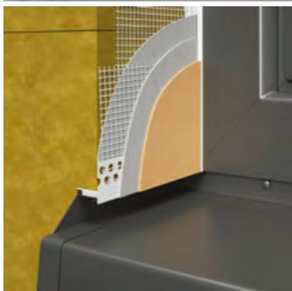
**LX-SPP window sill connecting bead** with glass fibre mesh and foam tape to ensure elastic connection of the plaster to the sill ending and to drain off the water from the reveals in the thermal insulation system - ETICS
