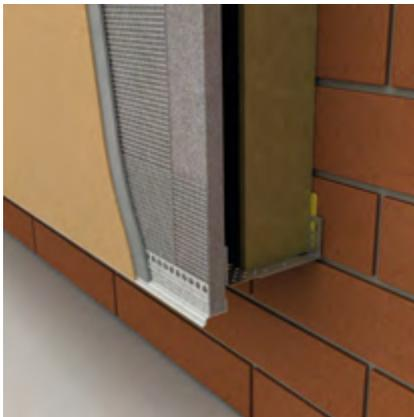
**LE-N drip bead** for facade boards of ventilated plastered facades
