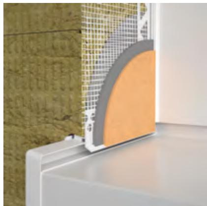
**LX-SPP FLEX window sill connecting bead** with invisible drip-edge (hidden under plaster), glass fibre mesh and foam tape to ensure elastic connection of the plaster to the sill ending and water drainage from the reveals in the thermal insulation system – ETICS
