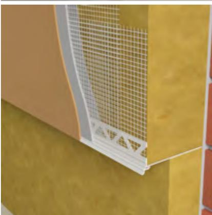
**LW-206 finishing and transition bead** with invisible drip edge and glass fibre mesh for the clean finishing of plasters and securing water drainage at the transition of different insulation thicknesses in ETICS. It is also the front part of the plastic set-up kit
