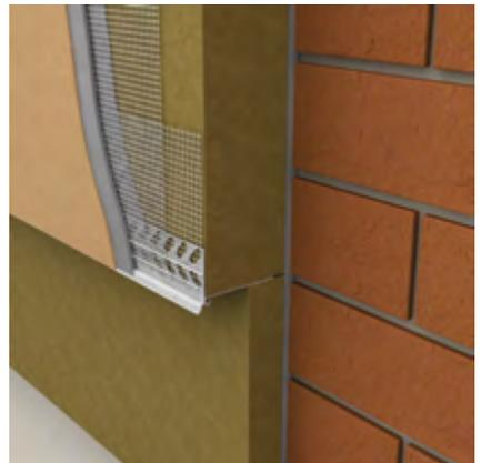
**LW-66-2 finishing and transition bead** with invisible drip edge and glass fibre mesh for the clean finishing of plasters and securing water drainage at the transition of different insulation thicknesses in ETICS. It is also the front part of the plastic set-up kit
