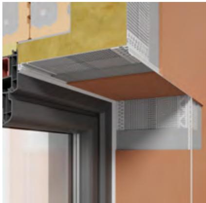
**LTNU window drip bead** with invisible drip-edge (hidden under plaster) and glass fibre mesh for finishing plasters and water drainage at the window heads in the thermal insulation system - ETICS. The bead can also be used as a balcony drip bead. The bead can also be at the bottom edge of the system where the LO base profile is not used for the insulation layer set-up
