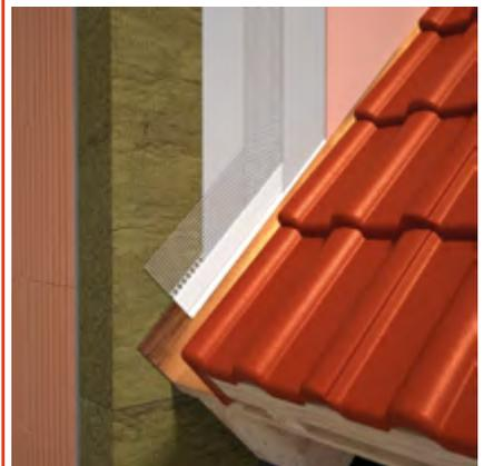
**LX-45-2 connecting bead** with glass fibre mesh for durable connection between metal flashing and plasters in the thermal insulation system - ETICS
