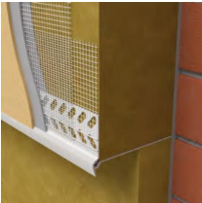
**LW-66 finishing and transition bead** with visible drip edge and glass fibre mesh for the clean finishing of plasters and securing water drainage at the transition of different insulation thicknesses in ETICS. It is also the front part of the plastic set-up kit
