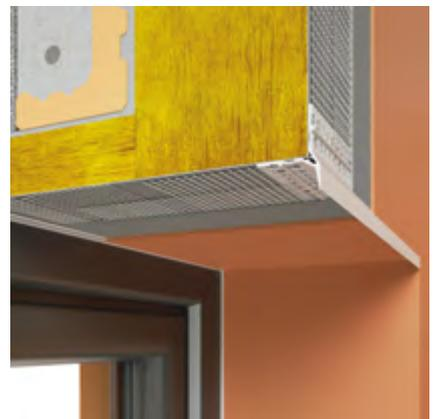
**VLTU window drip bead** with visible drip-edge and glass fibre mesh for finishing plasters and water drainage at the window heads in the thermal insulation system - ETICS. The bead can also be used as a balcony drip bead. The bead can also be at the bottom edge of the system where the LO base profile is not used for the insulation layer set-up
