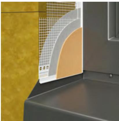
**LX-H flexible connecting bead** with mesh for window sills with invisible drip edge for creating flexible joint between plaster and ending of window sill in the thermal insulation system - ETICS. Suitable for connecting smaller metal flashings with plasters as well
