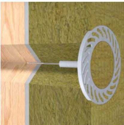
**Plastic anchor drive W with a screw** to be used for fixing thermal insulation boards in ETICS to wood and construction boards
