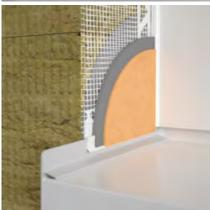
LX-H2 flexible connecting bead with mesh for window sills with invisible drip edge for creating flexible joint between plaster and ending of window sill in the thermal insulation system — ETICS. Suitable for connecting smaller metal flashings with plasters as well
