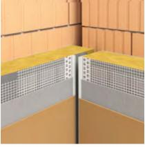
joining separate surfaces and forming a visible expansion joint in the thermal insulation system - ETICS
