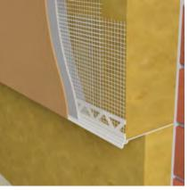
LW-L set-up profile to be used in the plastic set-up kit in the LW-206 finishing and transition bead with invisible drip LW-Z206 corner couplings for creation of internal and external edge and glass fibre mesh for the clean finishing of plasters corners of finishing beads LW-206 in the thermal insulation and securing water drainage at the transition of different system - ETICS insulation thicknesses in ETICS. It is also the front part of the plastic set-up kit
