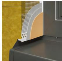
under plaster) and glass fibre mesh for finishing plasters and foam tape and changeable angle to ensure elastic connection of water drainage at curved window heads in the thermal insulation system - ETICS. The bead can also be used as a curved balcony drip bead. The bead can also be at the curved bottom edge of the system where the LO base profile is not used for the
