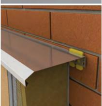
**LU-Z closing profile** with a drip edge used at the top of the insulation system to close the system and prevents water penetration. This profile is intended for use in details where connection to the wall is protected from rainwater.
