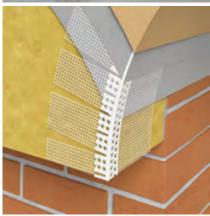
LK-KL2 arch corner bead for the protection of arch edges of LC-L stop bead with glass fibre mesh for finishing plasters a various radius in the thermal insulation system - ETICS
