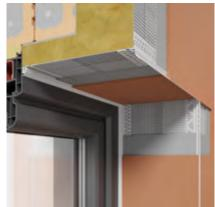
LTU window drip bead with invisible drip-edge (hidden under LTHU window drip bead with invisible drip-edge (hidden under plaster) and glass fibre mesh for finishing plasters and water drainage at the window heads in the thermal insulation system - ETICS. The bead can also be used as a balcony drip bead. The bead can also be at the bottom edge of the system where the LO base profile is not used for the insulation layer set-up
