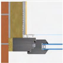
LS2-FLEX COLOR 2D window reveal bead with a protective LS2-30 plus 2D window reveal bead with a protective lip and LS3-200 3D window reveal bead with flexible loop and glass
