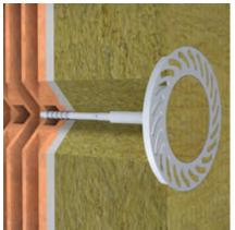
Plastic anchor eco-drive W 8 with an anchor plate Plastic anchor drive W with a screw to be used for fixing Plastic anchor drive S with a screw for counter sunk diameter of 110 mm and a preassembled metal screw for counter-sunk fixing thermal insulation boards in the thermal insulation system - ETICS
