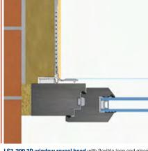
lip and glass fibre mesh for elastic connection between the window or door frame and plaster in the thermal insulation
