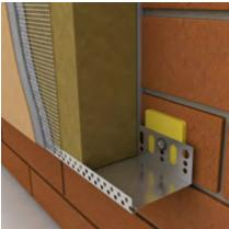
LO base profile (also known as a starter track or base rail) incl. a drip edge used for horizontal set-up of thermal insulation boards in the thermal insulation system - ETICS
