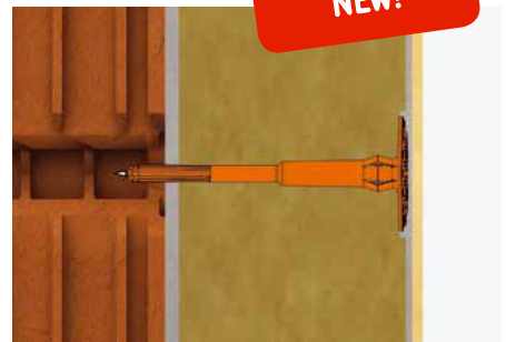
Plastic anchor PTH-EX 8 with a metal pin for fixing thermal insulation boards in the thermal insulation system – ETICS
