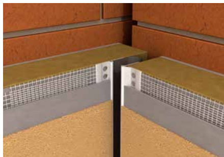
LD-LS corner expansion bead with glass fibre mesh for joining separate surfaces and forming a visible expansion joint in the thermal insulation system – ETICS
