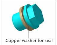
Screw up the oil drainage bolt before filling-up new oil, remove and well keep the oil drainage tube, then lock up the oil drainage switch on the case.
