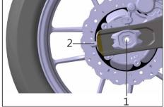
Fastening torque of adjusting nut: 14NM Fastening torgue of rear wheel axle: 95NM
