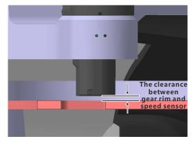
The gap between gear rim 1 and speed sensor 2:0.2mm~1.2mm
