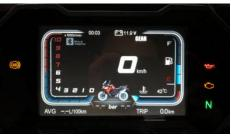
Rotation speed: The rotation speed of the engine. (r/min-Rotation/Minute-----The rotation turning circles each minute of crankshaft)
