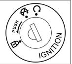
There are three positions on the ignition switch: "Q" means the ignition circuit connected which could be started anytime and all the functional circuits are connected. The key is unable to be removed when in this position. "Q" means the ignition switch circuit cut off which is unable to be started. The key could be removed when in this position.
