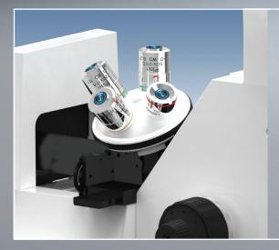
A slide-in polarizing kit with built-in polarizer/ analyzer fits seamlessly beneath the objective turret for user convenience. The kit comes equipped with a rotating polarizer for 360 degrees of light extinction. The LABOMED MET 400 is a workhorse tabletop metallurgical microscope that takes on a compact and highly durable form, making it the ideal candidate for daily inspection of heat-treated and stress-tested metals, glass, plastics, and chemicals.
