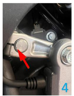
For correctly adjust shifting is neccessary the original (OEM) spacer/cogwheel turned down by 2 cogs/teeth. The dot stamped on the shift axis must be here as shown in pic. 4. Further adjustment is achieved by the rod shift.
