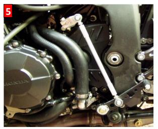
**Right side installation** The right side is mounted in the same way as the original (OEM) rearset.
