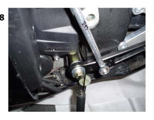
The shift shaft joint is needed to be dismantled and turned around (pictures A,B,C)
