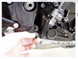
Loose the nut and pull out the bolt on the left side of the bike.
