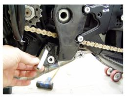
Put the spacer supplied in PP Tuning kit on the thread which is sticking out and tighten up.
