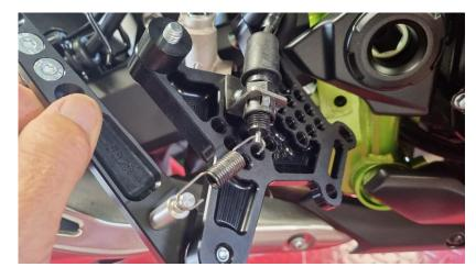
Brake pump must be placed perpendicularly on the brake pedal. For adjustment and right step can be moved by the brake cylinder to the left, see red arrow on the picture 4. Last step of the installation is adjusting the correct function of the brake light according to picture 5.
