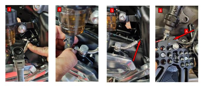
Now you have to insert the brake sensor behind the main plate (arrow A, pic, 6) and tighten M6 screw very lightly, which will secures the sensor against loosening. The brake sensor is plastic so tighten it gently! Secure the screw by adhesive for screws for example LOCTITE 243, or other similar.
