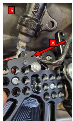
Now you have to insert the brake sensor behind the main plate (arrow A, pic. 6) and tighten M6 screw very lightly, which will secure the sensor against loosening. The brake sensor is plastic so tighten it gently! Secure the screw by adhesive for screws for example LOCTITE 243, or other similar.
