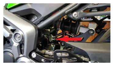
The brake fluid holder has to be mount according to picture nr. 3. Don't forget put under the lower screw M8 washer (see arrow on the picture nr.4). Without this washer the brake master cylinder will be crookedly mounted!
