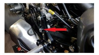
After replacing the brake hose is neccesary fit also brake sensor for rear brake light. (picture nr.5)
