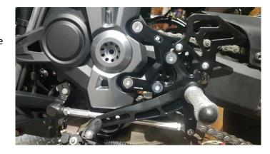
Right side installation At right side is necessary exchange ABS brake hose (is part of the packaging). Follow the pictures nr. 2
