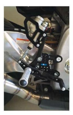
Right side installation Right side is different from serial version in assembly of brake pump. Is necessary turn brake pump about 180° (see photo 2.+3.)
